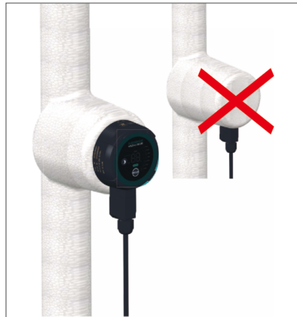
(Heat insulation of the pump body)
